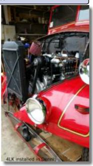
drawn is 21A, we employed a modern 90A alternator, belt driven from the crankshaft pulley. As far as we know neither the ZF nor the 4LK has ever been
